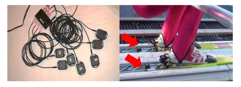
Fig. 1: Data logger connected to USB for charging (left). IMU installed on skis (right).
