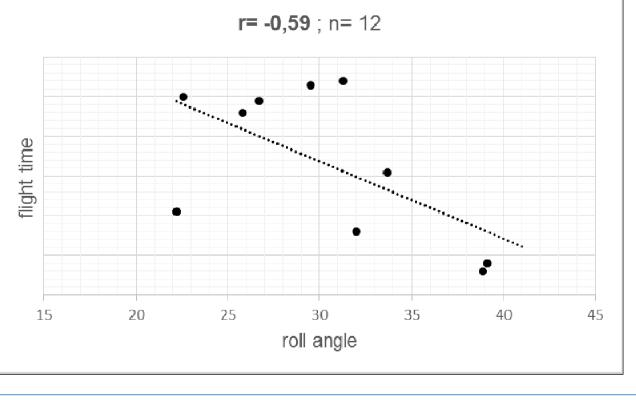
Fig. 4: Roll angle correlated to flying time. Relevant influencing factors (pitch angle, in run speed, outer conditions) are assumed to be nearly constant.
